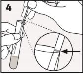
ALIGN: Lower the swab into the tube until the visible scoreline on the shaft is lined up with the tube rim. The bud of the swab should not be submerged into the liquid prior to breaking the shaft.
